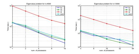
**Fig. 3.** Scalability of the Symmetric Eigenvalue Solver routines in ScaLAPACK (pdsyev) with a matrix of size 4,000 (*left*) and one of size 12,000 (*right*). Four different methods for the tridiagonal eigensolve have been tested: the BX (pdsyevx), QR (pdsyev), DC (pdsyevd) and MRRR (pdsyevr).
