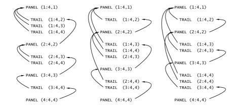
Fig. 1. Different possible factorization schemes: right-looking with no lookahead, right-looking with a lookahead of 1, left-looking (right-looking with maximum lookahead). Arrows show data dependencies.
